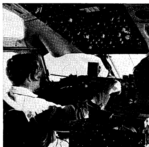
Fig. 3 Overhead installation of collimator with glareshield mounted reflector in DC-9.
